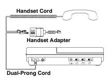
**Note:** Plug the dual-prong cord's plug into the larger modular jack and the handset cord's plug into the smaller jack.
